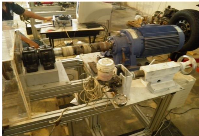
Figure 2 Drag type brake dynamometer used for the test
