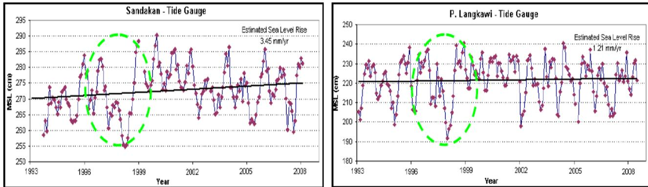
Figure 7 Positive linear trend of sea level rise at Sandakan and Pulau Langkawi tide gauge stations<sup>36</sup>
