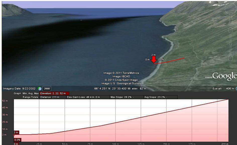
Figure 3 Coastal slope measurement using Google Earth<sup>24</sup>
