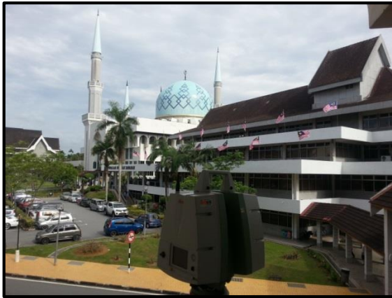
Figure 11 3D topography measurement using TLS.
