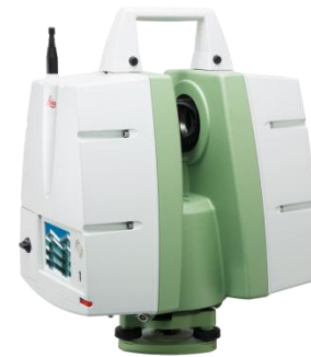
Figure 3 Leica ScanStation C10 scanner used in the experiments.
