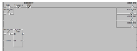
Figure 7 PLC ladder diagram example
