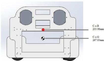
Figure 6 ROV center of buoyancy (C.o.B) and center of gravity (C.o.G)
