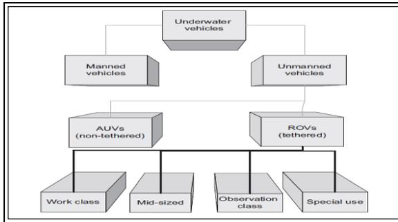
Figure 1 Underwater vehicles and ROVs
