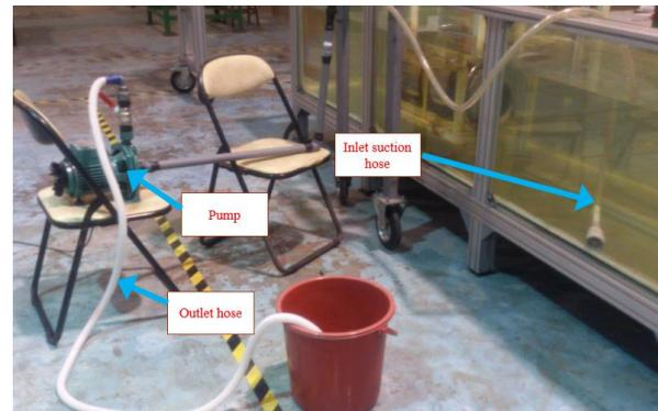
Figure 11 Cleaning set-up
