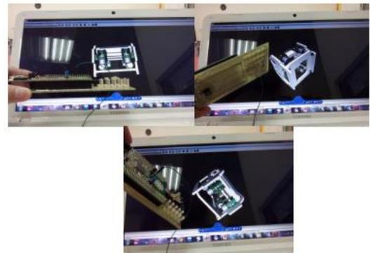
Figure 19 Actual Simulation of ROV movement with IMU
