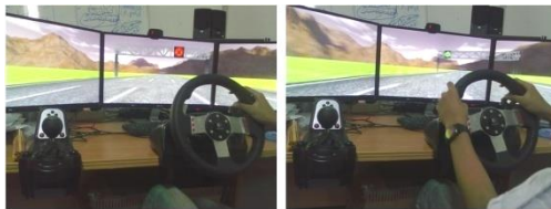
Figure 1 The modified OpenDS Driving Simulator with signs to reduce the car's speed (left) and to change lanes (right)
