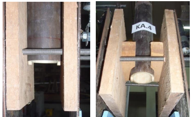
Figure 11 Failure mode in the connection system in tension (a) Without wooden clamps(NKA); (b) with wooden clamps (KA)
