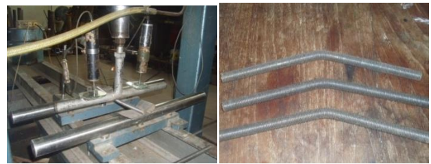
Figure 10 Testing of bending moment of bolt
