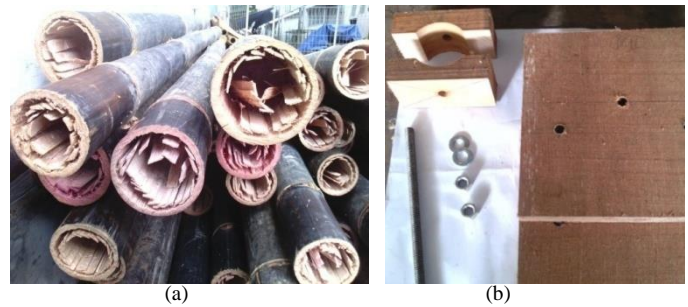
Figure 7 Material of specimen (a) bamboo (b) bolt with a diameter of 12.2 mm, wooden clamps and wood board
