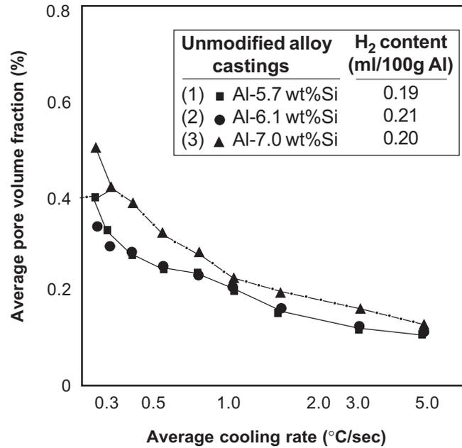
**Figure 5** Average pore volume fraction as a function of average cooling rate for alloys with silicon contents of 5.7%, 7%, and 8.1 wt % [14]
