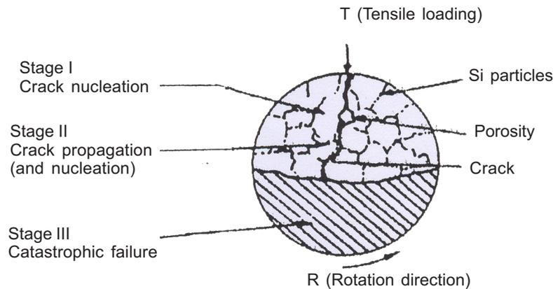
**Figure 9** Fatigue failure of Al-7Si-0.3Mg alloy [21]
