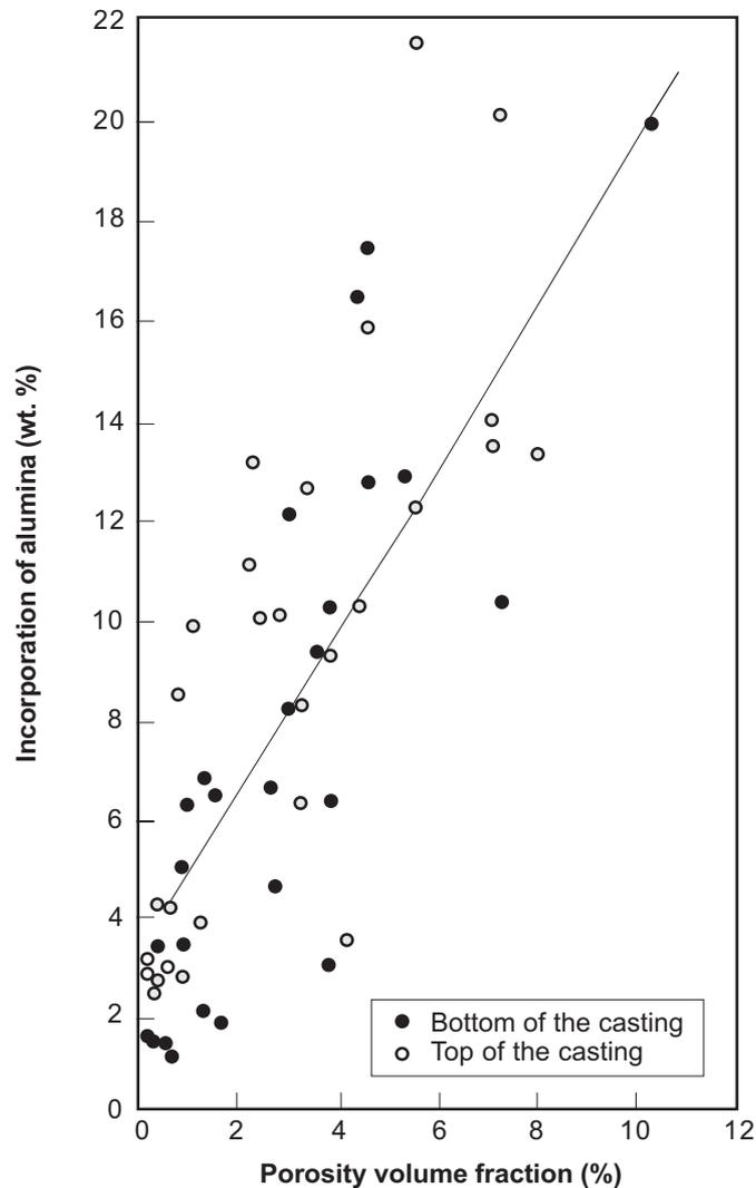
**Figure 2** Variation of porosity, with alumina content in cast Al-Al<sub>2</sub>O<sub>3</sub> composites [13]
