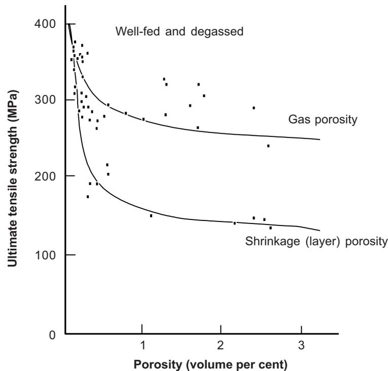
**Figure 10** The reduction in UTS of an Al-11.5Mg alloy by dispersed porosity and by layer porosity [26]
