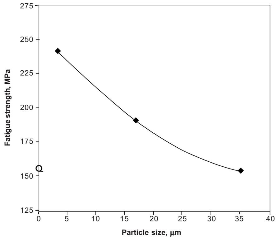
**Figure 12** Effect of particle size on fatigue strength in 2124/SiC/20p (at 10 cycles,  $R=-1$ ) [27]
