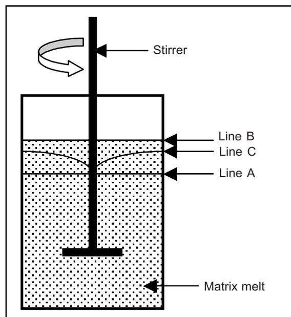
**Figure 6** The effects of vortex formation on the surface of a matrix melt [4]
