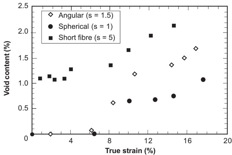
**Figure 1** Void content as a function of tensile strain for composites containing three types of  $Al_2O_3$  reinforcements of a volume fraction of 10% [12]
