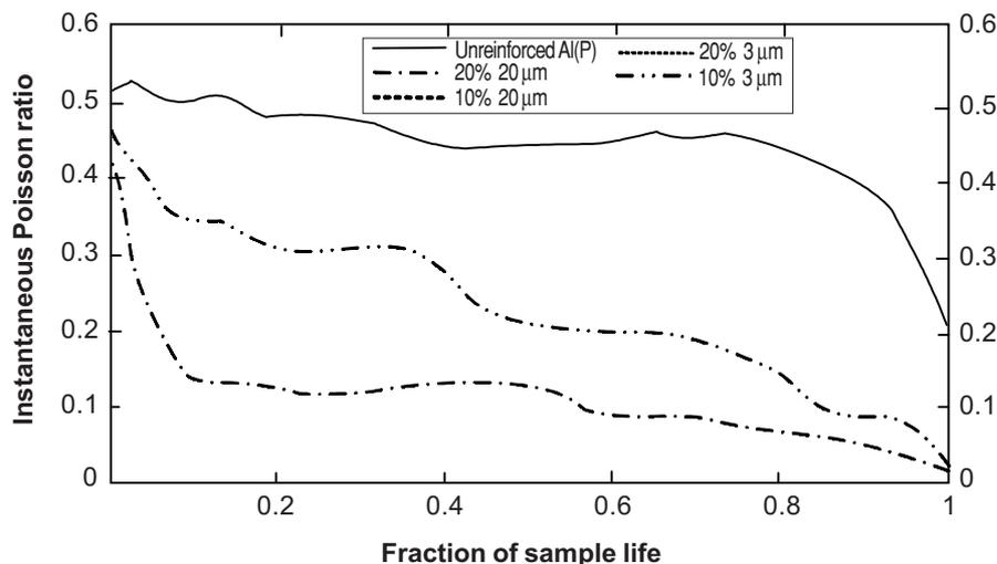
**Figure 8** Instantaneous Poisson ratio as a function of specimen life for SiC reinforced Al composites [11]
