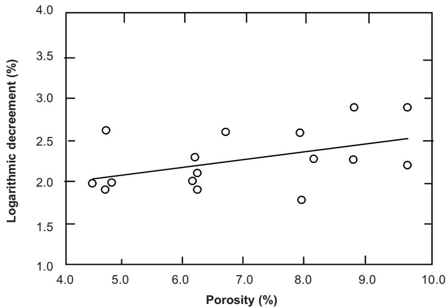
**Figure 13** Relationship between damping capacity and porosity for 6061Al [28]
