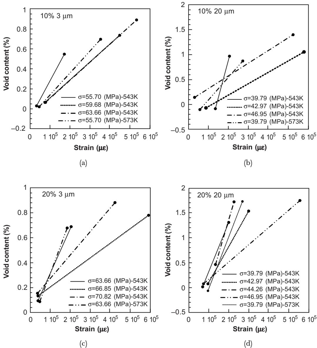
**Figure 11** Void content of the specimen for SiC particulate reinforced Al composites as a function of applied stress [27]
