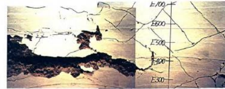
Figure 18 Concrete crushing inside face of circular hollow pile [13]
