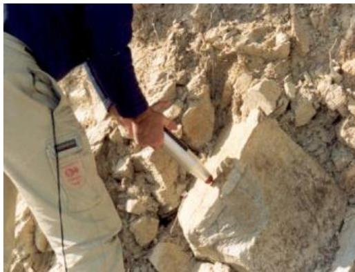
(c) Surface hardness test using rebound hammer
