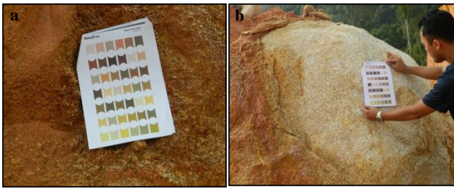
Figure 5 Identification of rock colour; a) Rock colour chart, b) Determination of boulder's colour
