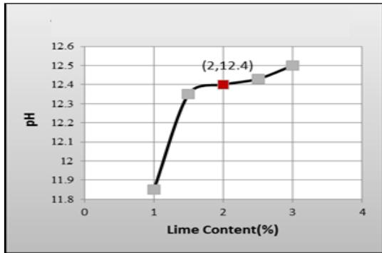
Figure 1 Results of the ICL test for Kaolin clay soil
