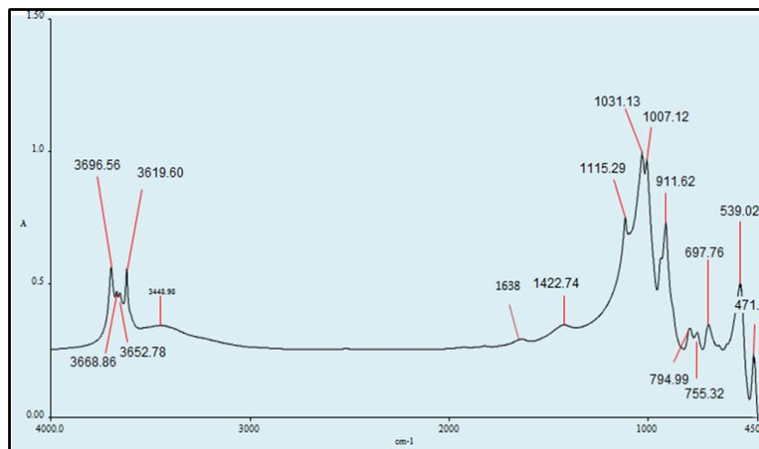
Figure 8 FTIR Spectra for natural Brown Kaolin clay soil
