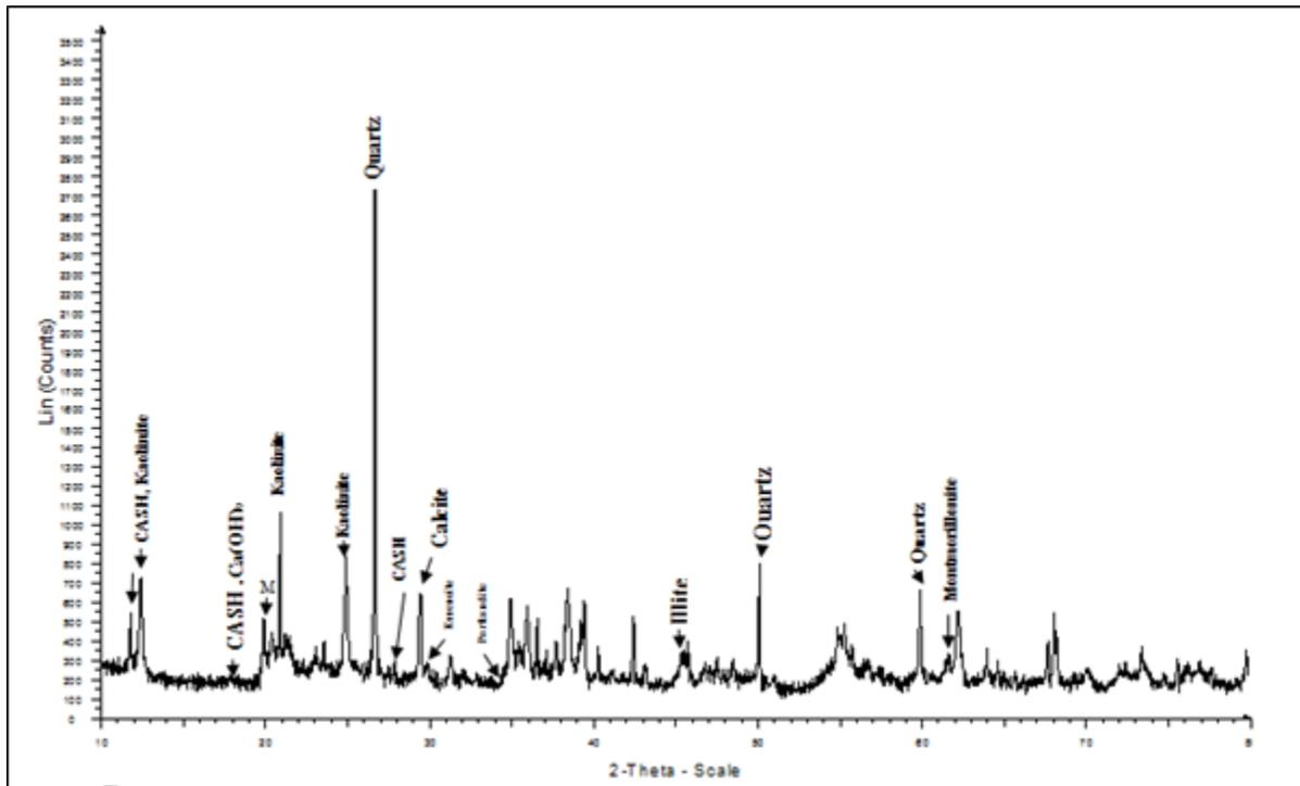
Figure 6 XRD for Kaolin clay samples treated by 10% cement at 200 days curing time
