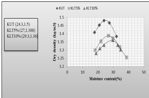
\* KUT = Untreated Kaolin, KLT = Lime-treated Kaolin
