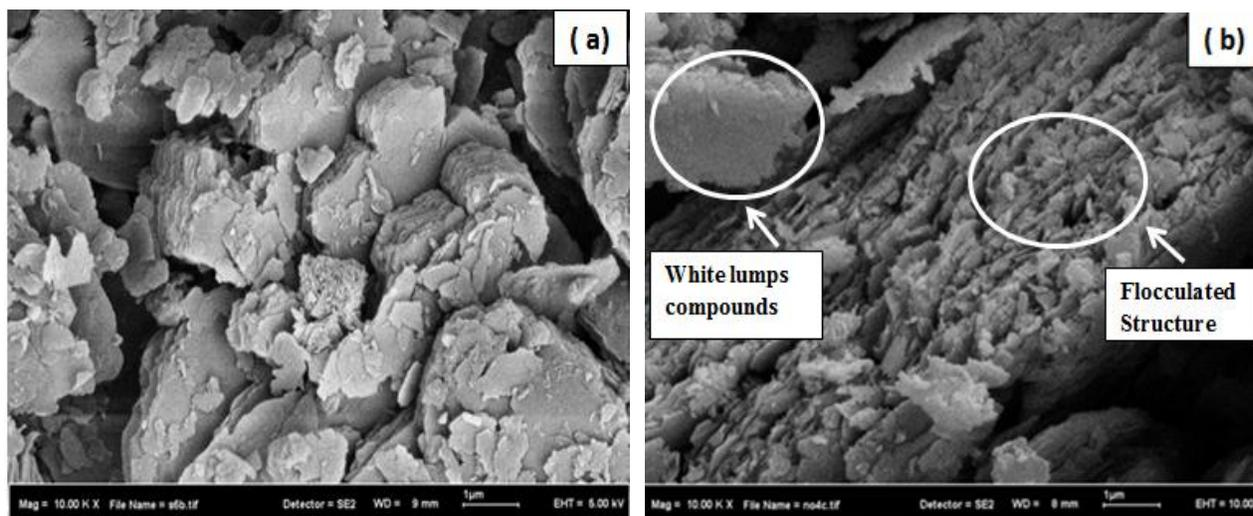
**Figure 7** FESEM image of (a) untreated Kaolin clay soil and (b) 10% lime treated Kaolin clay after at 200 days curing time at magnification of X10.000.
