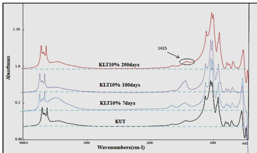
Figure 9 FTIR spectrums of natural and lime treated Kaolin Clay at different time intervals
