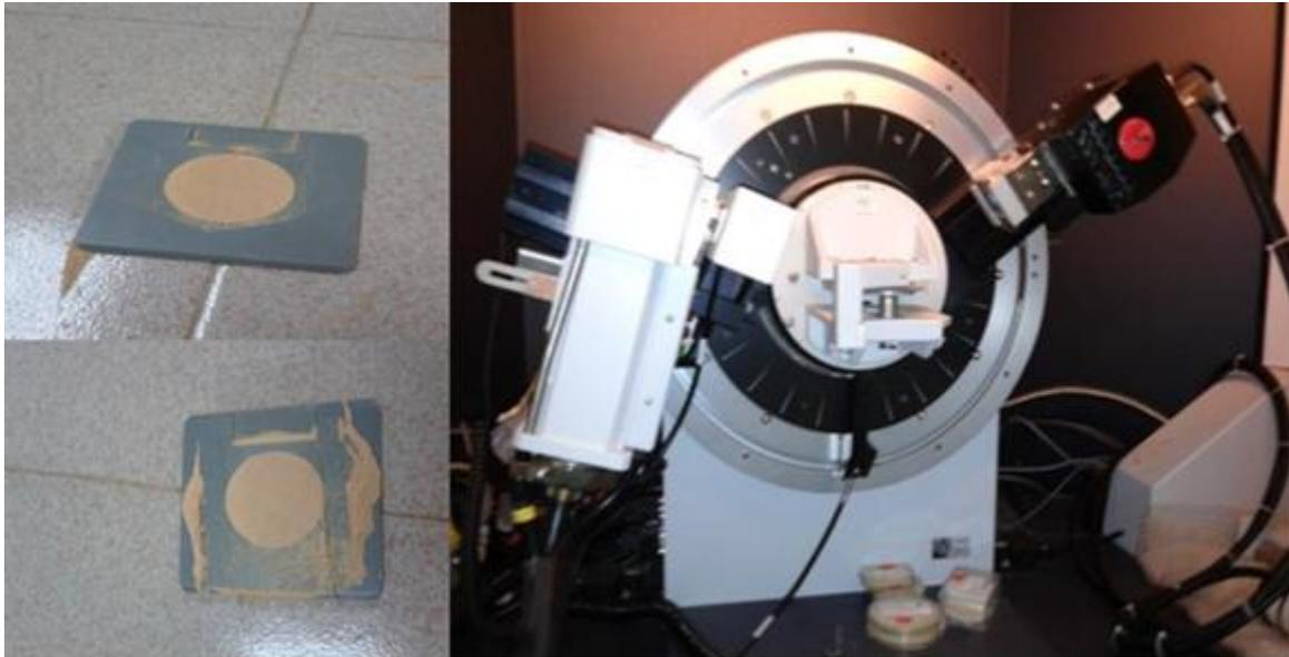
**Figure 4** Samples preparation and apparatus of XRD-Diffraction test
