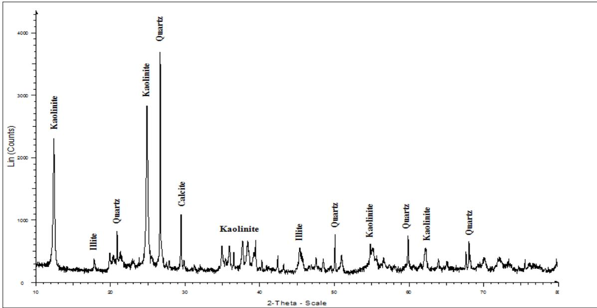
Figure 5 XRD of untreated Kaolin clay soil
