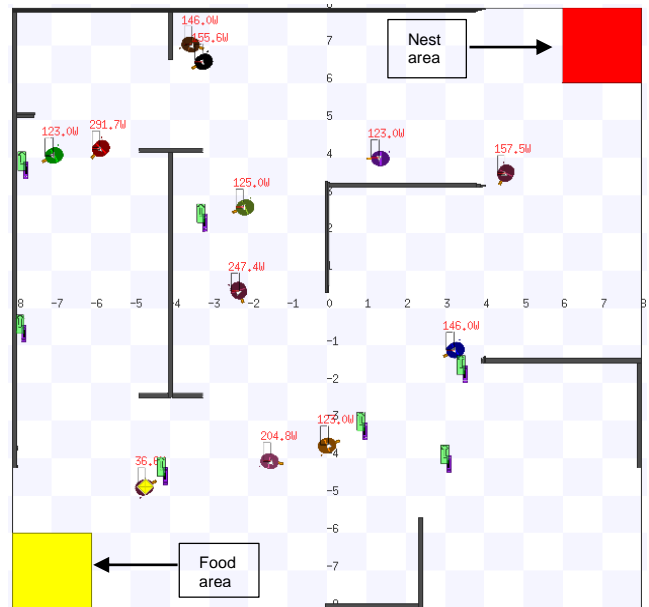
Figure 2 the arena with foraging robots with their energy level shown moving in environment where power stations are deployed
