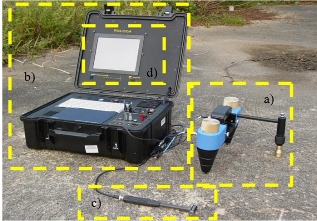
Rajah 1 Sistem PiScanner. a) PiScanner Probe, b) POLCCA, c) Penukul, d) PiScan Analyzer
