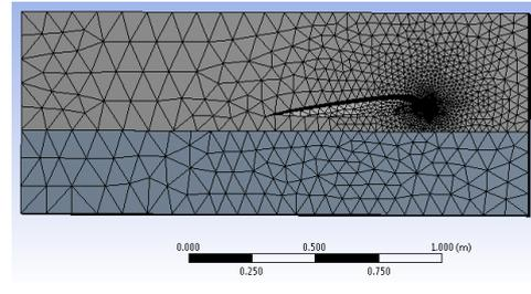
**Figure 20** Meshing on the outer wing and pontoon
