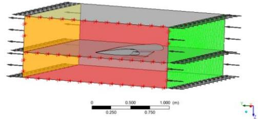
**Figure 21** Isometric on the outer wing and pontoon
