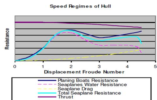
Figure 4 The resistance versus Speed<sup>7)</sup>
