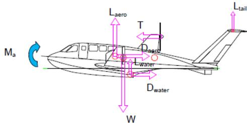
Figure 2 The forces distribution on the Wing in Surface Effect craft B type during hydro planing<sup>9)</sup>
