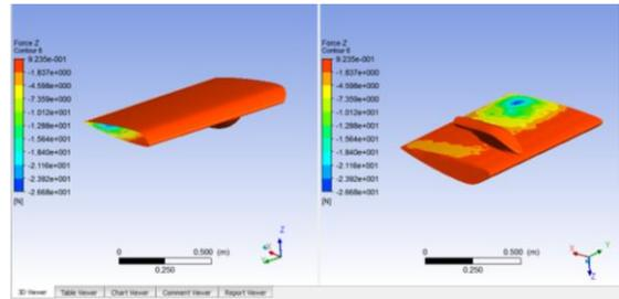
**Figure 28** The Force (Z lifting) distribution on the outer wing and pontoon
