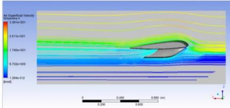
**Figure 24** The result of Air Velocity Streamline on the outer wing and pontoon
