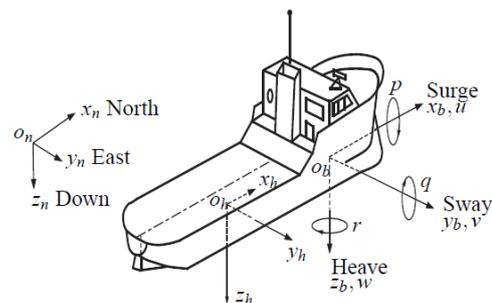
Figure 5 Notation and sign conventions for ship motion<sup>12)</sup>
