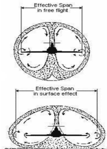
**Figure 1** The effective span during free flight and nearby surface effect<sup>[11]</sup>
