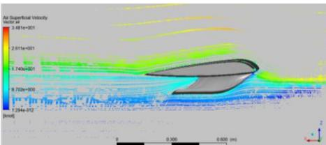
**Figure 26** The result of Air Velocity Vector on the outer wing and pontoon
