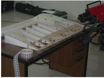
**Figure 16** The outer wing and pontoon with the marker during photo camera laser tracking process
