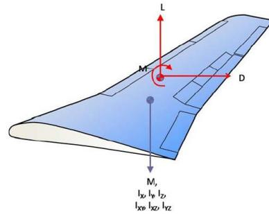
Figure 3 The lift, drag and moment of aerodynamic on the wing surface<sup>11)</sup>
