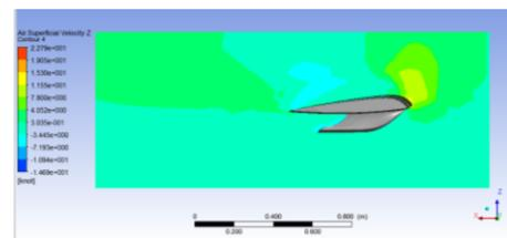
**Figure 22** The result of Air Pressure Distribution on the outer wing and pontoon
