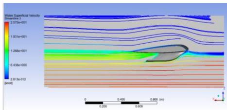
**Figure 25** The result of Water Velocity Streamline on the outer wing and pontoon
