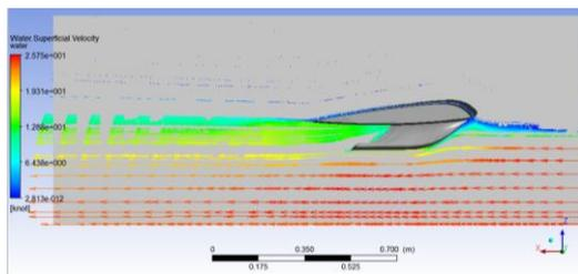
**Figure 27** The result of Water Velocity Vector on the outer wing and pontoon
