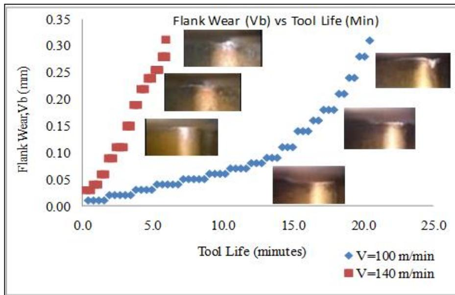
**Figure 5** Effect of cutting speed on tool life with feed rate of 0.15 mm/rev and depth of cut 0.35 mm
