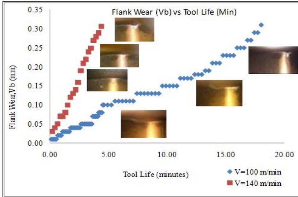
**Figure 4** Effect of cutting speed on tool life with feed rate of 0.20 mm/rev and depth of cut 0.35 mm.
