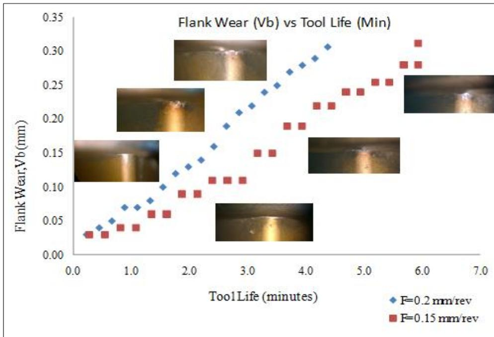
Figure 3 Effect of feed rate on tool life with cutting speed of 140 mm/min and depth of cut 0.35 mm
