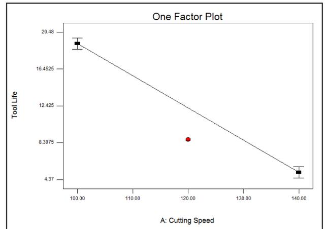
**Figure 7** One factor plot of cutting speed versus tool life
