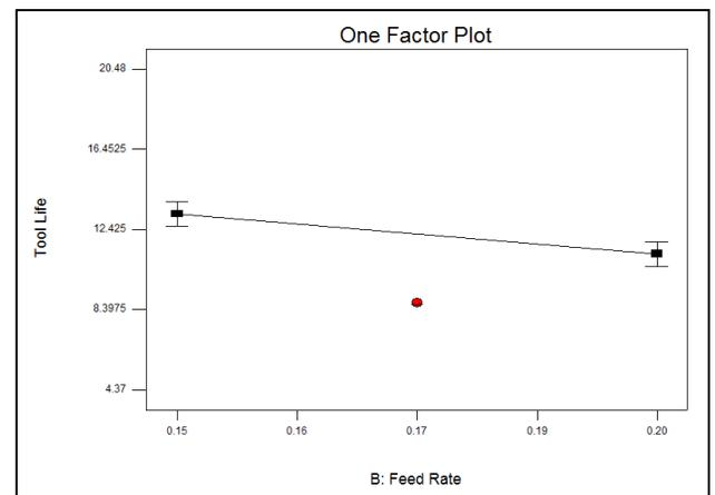
**Figure 8** One factor plot of feed rate versus tool life
