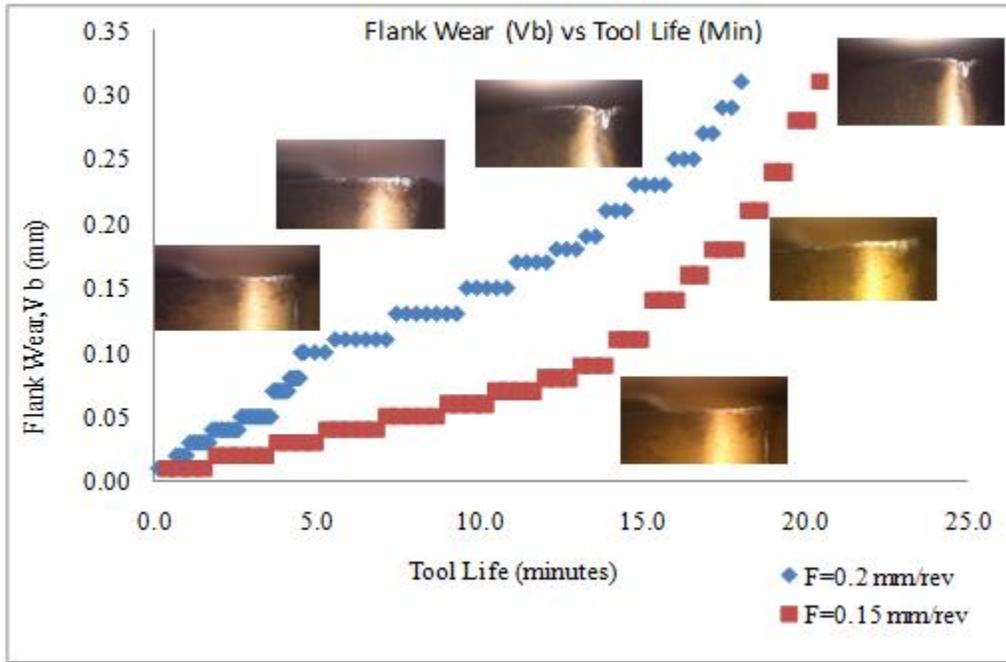
Figure 2 Effect of feed rate on tool life with cutting speed of 100 mm/min and depth of cut 0.35 mm
