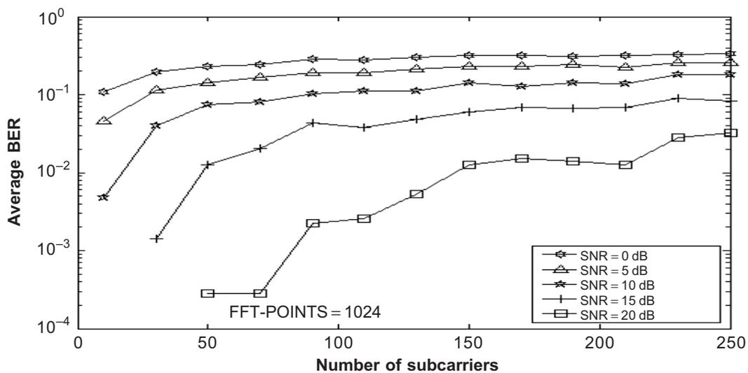
**Figure 2** BER versus number of subcarriers for 16-QAM in AWGN channel at different SNR
