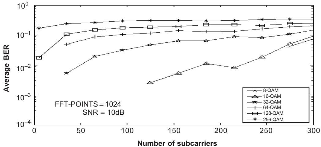
**Figure 7** BER versus number of subcarriers for M-QAM OFDM over AWGN channel at SNR = 10 dB
