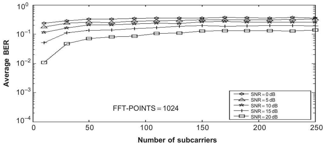
**Figure 3** BER versus number of subcarriers for 64-QAM OFDM in AWGN channel at different SNR
