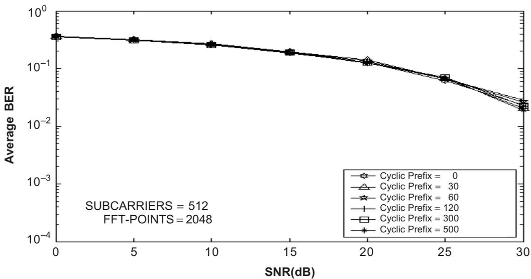
**Figure 9** BER versus SNR for 64-QAM over AWGN channel utilizing different length of cyclic prefix
