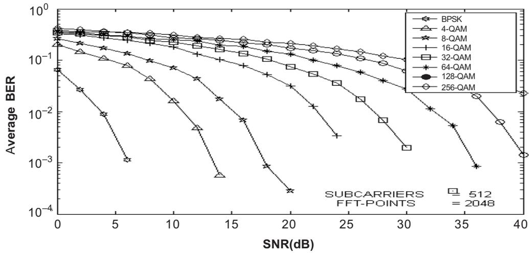
**Figure 6** BER versus SNR for M-QAM OFDM in AWGN channel with FFT-points = 2048
