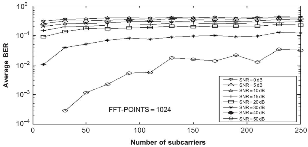
**Figure 4** BER versus number of subcarriers for 256-QAM OFDM in AWGN at different SNR
