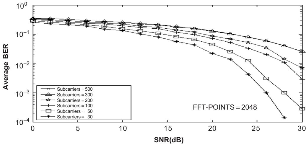
**Figure 8** BER versus SNR for 64-QAM over AWGN channel using different number of subcarriers
