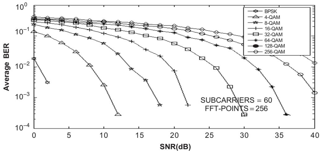
**Figure 5** BER versus SNR for M-QAM OFDM in AWGN channel with FFT-points = 256
