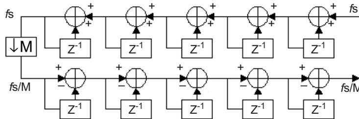
**Figure 12** Comb filter implementation architecture
