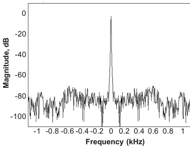
**Figure 15** Experimental performance of DECT digital front-end
