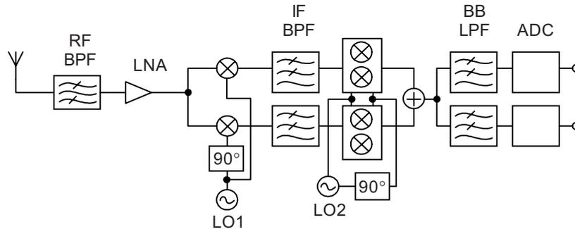
**Figure 5** Wideband IF double conversion architecture
