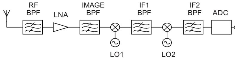
**Figure 5** Wideband IF subsampling architecture
