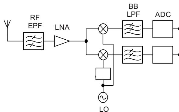
**Figure 3** Direct conversion architecture
