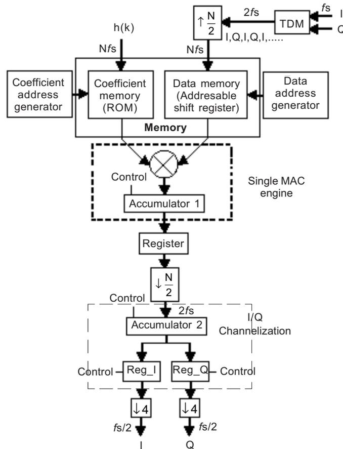
**Figure 13** Dual channel polyphase MAC FIR filter implementation architecture
