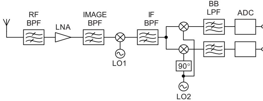
**Figure 2** Superheterodyne architecture
