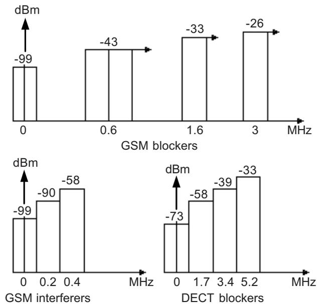
**Figure 9** GSM and DECT blockers and interferers specifications
