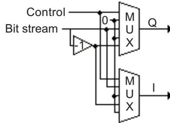
**Figure 11** I/Q downconversion implementation architecture
