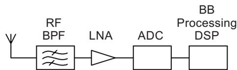
**Figure 1** The ideal software radio receiver
