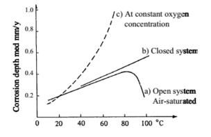
Figure 9 Corrosion of steel in water as a function of temperature [31]
