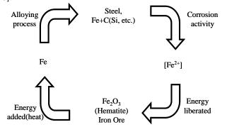
Figure 1 Refining-corrosion cycle
