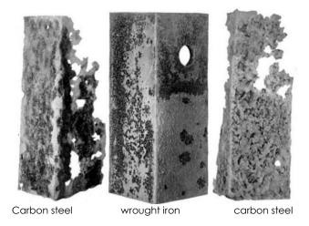
Figure 2 The unequal corrosion of different structural steels
