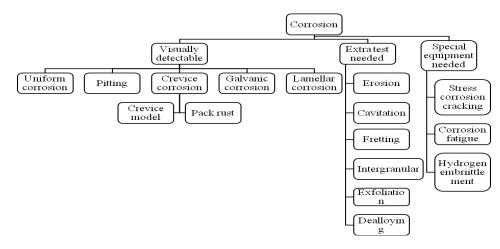
Figure 12 Various types of corrosion in different metals [31]
