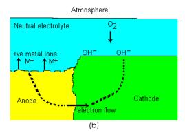
Figure 6 Schematic representation of galvanic influence on corrosion  $\left[10\right]$
