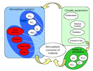
Figure 5 Environmental factors that affect metal corrosion [22]
