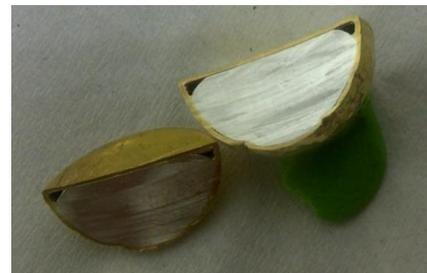
**Figure 4** Photograph of the earrings after being sectioned into two pieces
