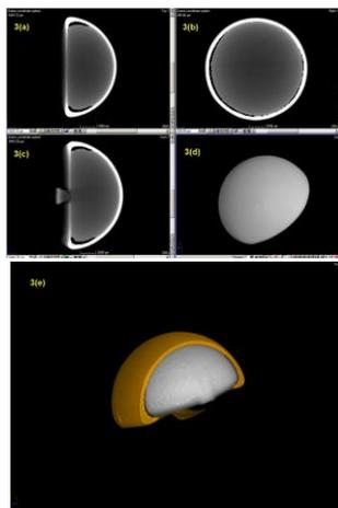
**Figure 3** Reconstructed X-ray computed tomography images (2D and 3D) of a fake gold ear-ring using dual energy approach of 140 kV and 225 kV. The images revealed that the ear ring is made of two different metals (outer layer of about 288-300 $\mu\text{m}$  thick is 22K gold and inner part is silver), and air voids are clearly be seen in certain locations between these two precious metals
