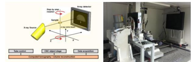
**Figure 2.** A schematic diagram (left) and a photograph (right) of a cone beam X-ray micro computed tomography system using a flat panel detector and a cone beam X-ray source.
