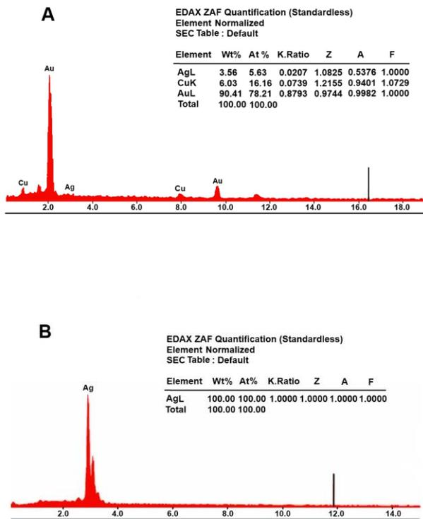
**Figure 5** Results of the SEM-EDX analysis of the sectioned surface after it has been polished and cleaned with distilled water. Spectrum in A represents elemental composition of the outer layer and spectrum in B corresponds to elemental composition of the inner part
