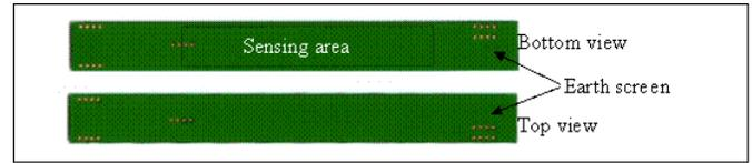
Figure 3 Sensing plate PCB
