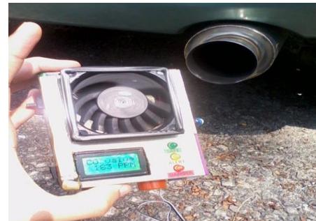
Figure 9 CO smart detector during a test using car fumes
