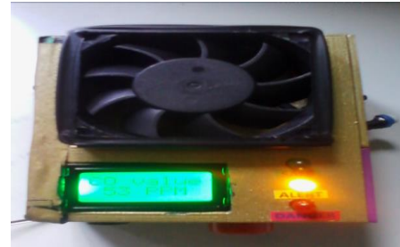
Figure 8 CO smart detector during a test in a room filled with cigarette smoke
