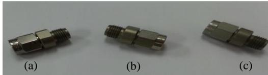
**Figure 9** Attenuators that used as device under tests (DUTs): (a) 3 dB (b) 6 dB and (c) 10 dB
