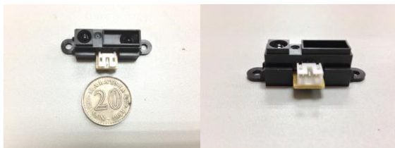
Figure 1 Top and side view of GP2D120 IR sensor
