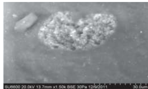
Figure 6 FE-SEM microstructure images of nanoclay modified binder [39]
