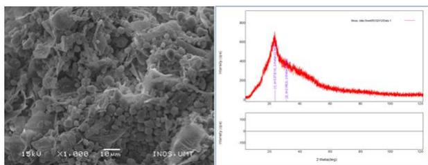
Figure 2b SEM Image and XRD Pattern for De-oiled Seed
