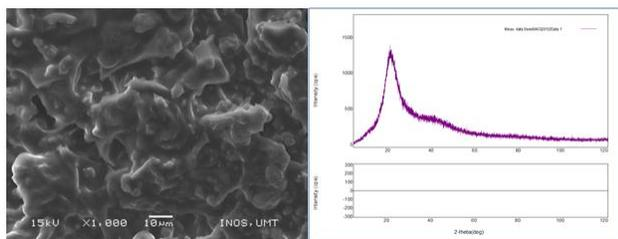
Figure 2a SEM Image and XRD Pattern for Untreated Seed
