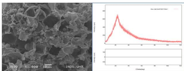
Figure 2c SEM Image and XRD Pattern for Treated De-oiled Seed
