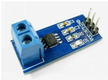
Figure 7 ACS 712 current sensor
