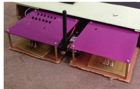
Figure 9 GSM modem installation
