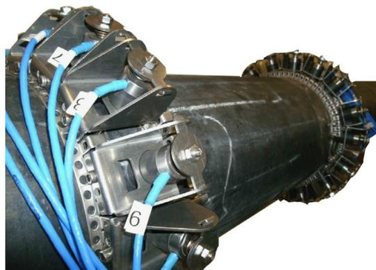
**Figure 7** An 8" diameter pipe is instrumented with two ring arrays each containing 16 EMAT transducers [34]
