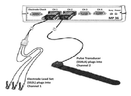
Figure 1 Experimental Setup For ECG And PPG Recordings [18]
