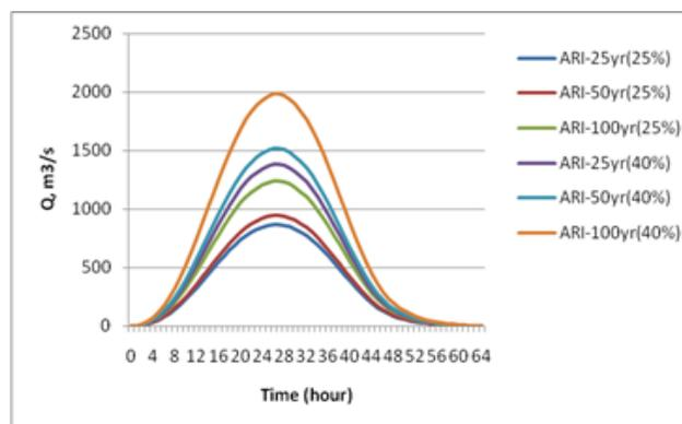
**Figure 3** Generated hydrograph for Wadi Alaqiq for 25% and 40% imperviousness using Arizona formula
