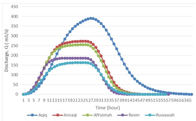
**Figure 4** Simulated hydrograph for 100 years at sub-catchment of Wadi Alaqiq (25% imperviousness)
