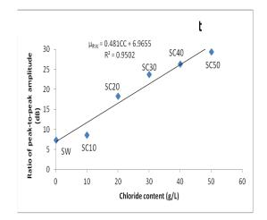
Figure 7 Peak-to-peak attenuation of reflected waves,  $\mu_{DW}$ , on chloride
