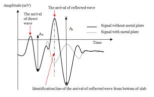
Figure 3 Typical time-domain plot of GPR waves
