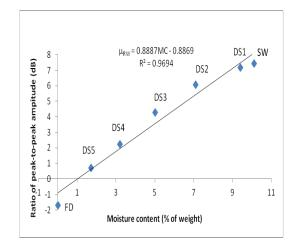
Figure 4 Peak-to-peak attenuation of direct waves,  $\mu_{DW}$ , on moisture
