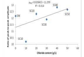
Figure 6 Peak-to-peak attenuation of direct waves,  $\mu_{DW}$ , on chloride
