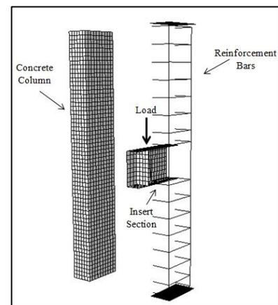
**Figure 2** Parts showing concrete column, reinforcements, and steel section
