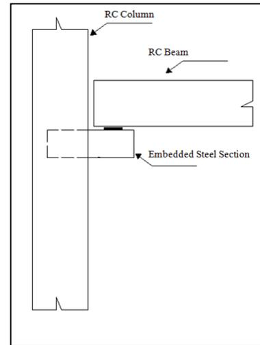
**Figure 1** A Typical reinforced concrete connection with embedded steel section
