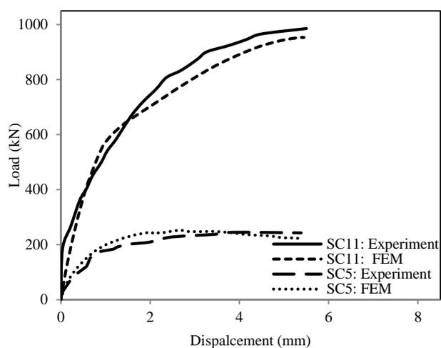
Figure 3 Comparison between finite element results and test results
