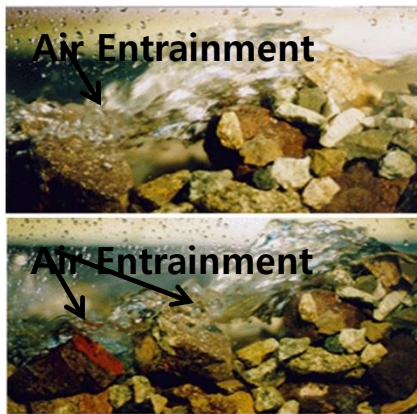
Figure 12 Air entrainment behind trailing edge of gravels
