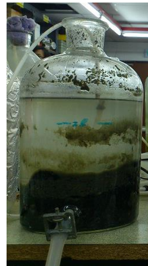
Figure 1 Lab-scale attached-growth SBR with additional biomass
