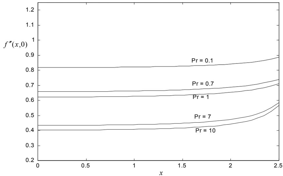
**Figure 3** Variation of the surface shear stress ( $f''(x,0)$ ) with  $x$  for sinusoidal variation in wall temperature and various Prandtl number,  $Pr$
