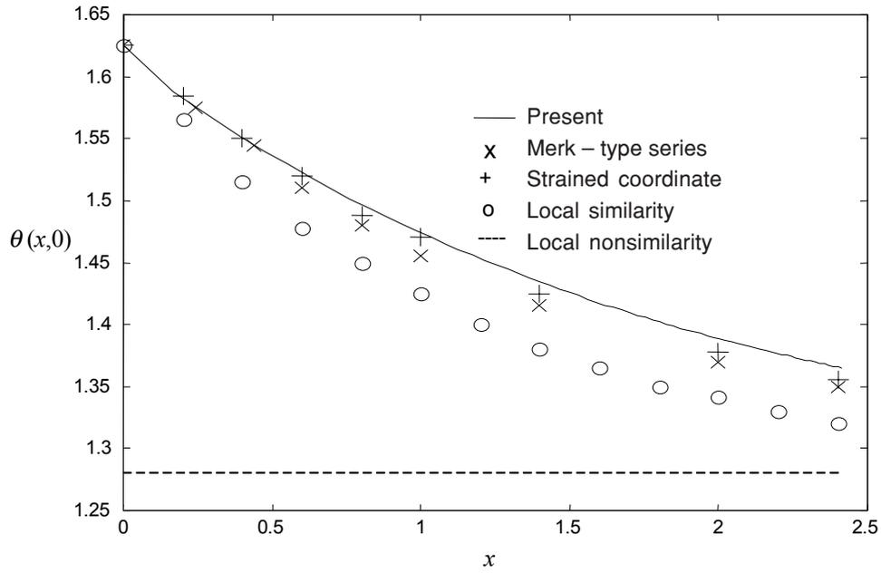
**Figure 6** Comparison of dimensionless temperature for exponential variation in surface heat flux ( $Pr = 0.7$ )
