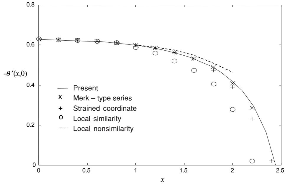
**Figure 2** Comparison of dimensionless temperature gradient for sinusoidal variation in wall temperature ( $Pr = 0.7$ )
