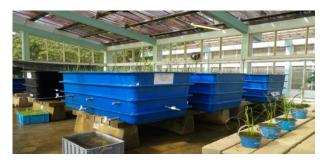
Figure 3 A pilot scale reed bed with sub- surface flow system
