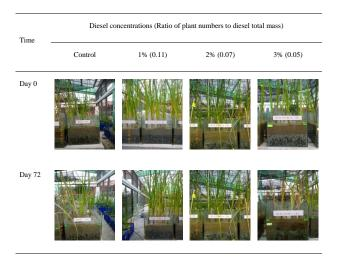
Based on the preliminary and phytotoxicity tests, we considered a minimum ratio of plant number to the total mass of 0.05 to determine diesel concentration in pilot reed bed run. Therefore, 0.1, 0.175 and 0.25% diesel concentrations with respective ratio of 0.11, 0.07 and 0.05 (Table 1) were selected to evaluate the performance of pilot reed bed to phytoremediate diesel.
