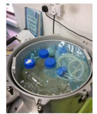
Figure 3 Sterilization process in an autoclave at a pressure of 1.2 x  $10^4$  Mpa
