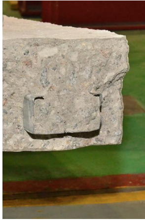
Figure 5 Tearing of shear connector
