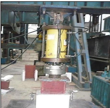
Figure 3 Push-out specimen under testing
