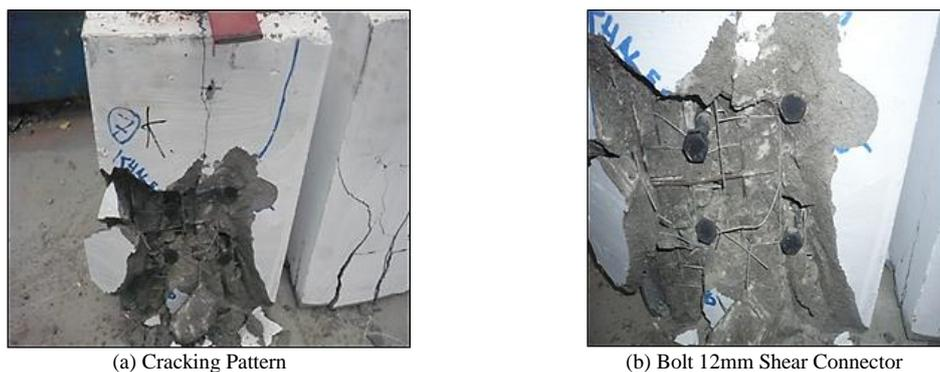
Figure 6 Crushing failure mode in ferrocement jacket
