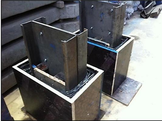
Figure 2 Preparation of CFS and wire mesh layers as column jacket
