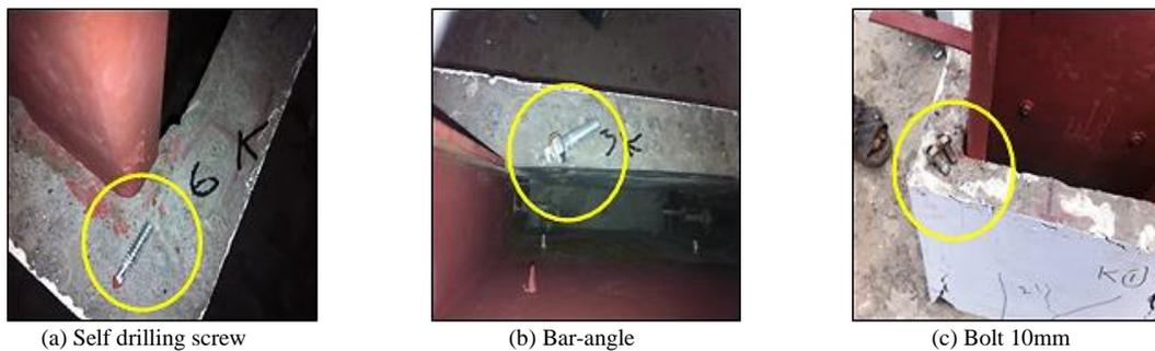
Figure 5 Failure modes of shear connectors
