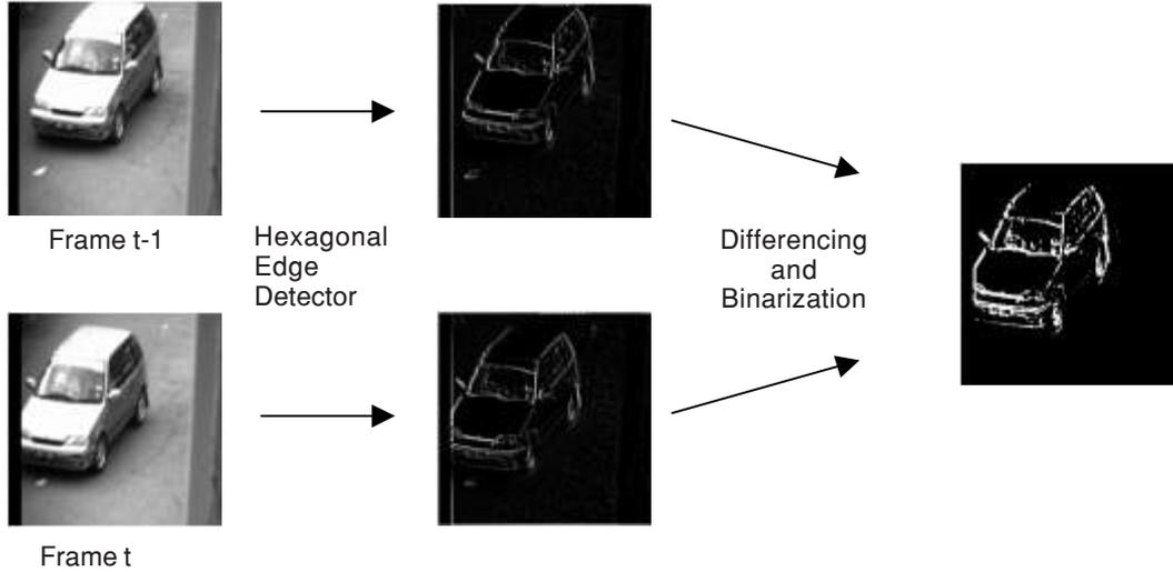
**Figure 2** Moving edges extraction process
