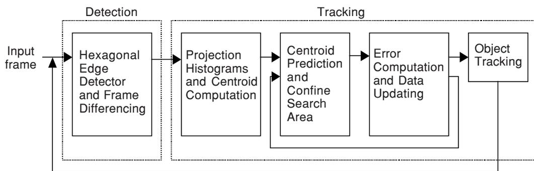
**Figure 1** The proposed detection and tracking algorithm
