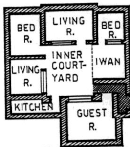
Figure 7. shows a simplified plan of Damascene traditional houses. Notice the shape of the entrance that forms the Medkal, private zone
