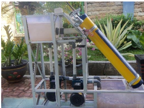
Figure 2 Turbine screw experimental apparatus
