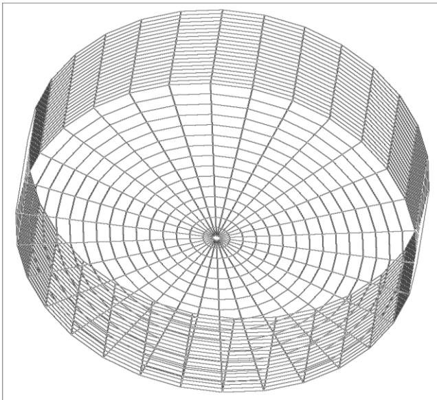
**Figure 7** Meshing for round shape FPSO model
