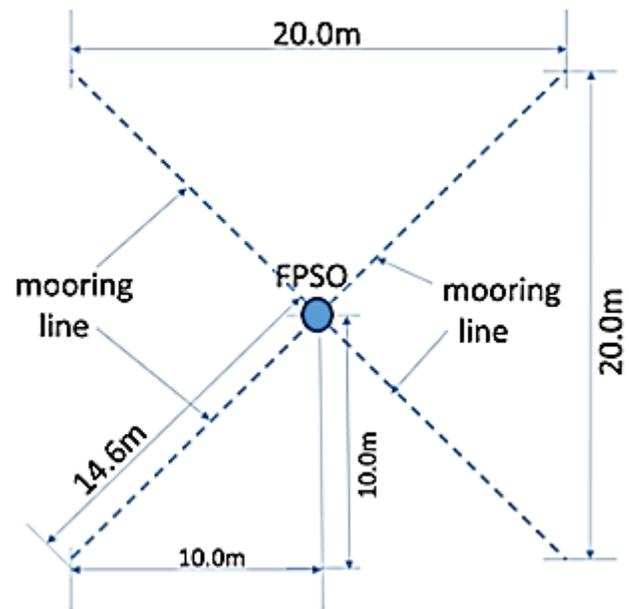
**Figure 3** Arrangement of mooring lines and anchor in wave basin
