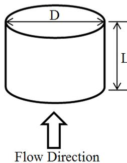
Figure 1 Dimension of vertical cylinder and flow direction
