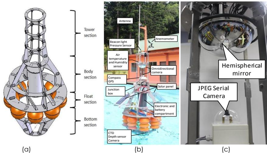
Figure 2 (a) MIOOS buoy structure (b) Sensor placements (c) Omni-directional camera
