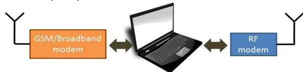
Figure 4 Ground station block diagram
