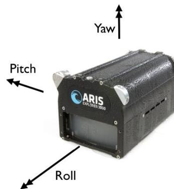
Figure 5 Three axes of the acoustic camera
