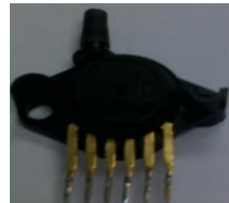
Figure 3 MPX4250AP CASE 867B-04 with pin configurations
