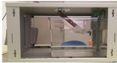
**Figure 5** Single link underwater robot manipulator
