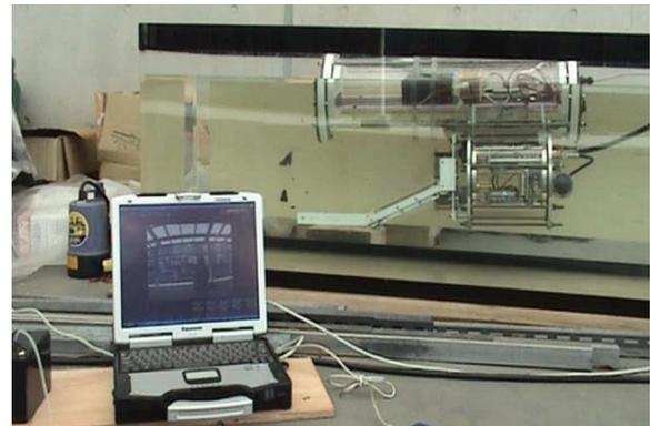
Figure 3 Underwater manipulator tap water experiment [3]
