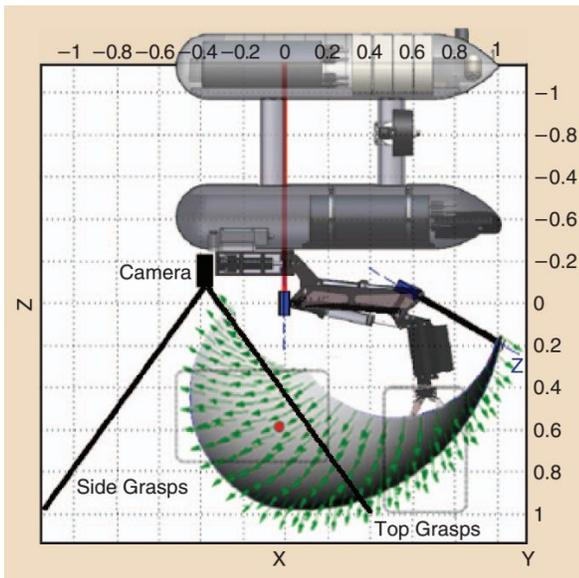
Figure 1 CSIP underwater robotic arm [1]
