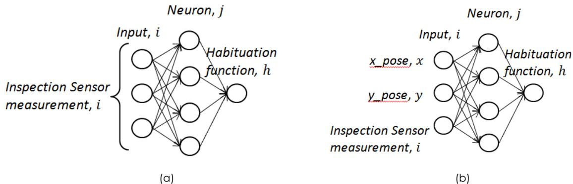
Figure 1 (a) usual HSOM network with all input associated to inspection sensor measurement. (b) HSOM network with spatial information as its input.
