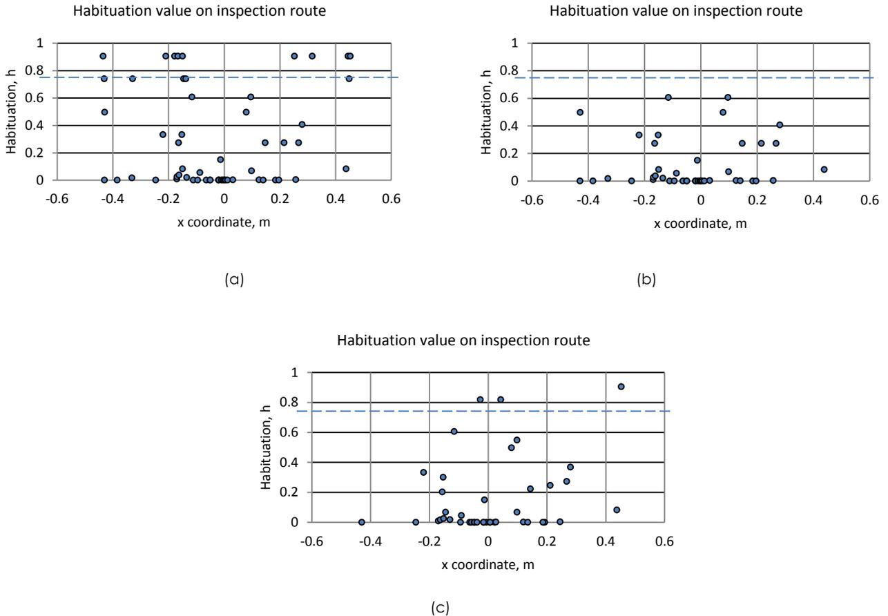
**Figure 6** (a) After 18 runs at learning rate = 0.01, with neighboring habituation function turned on (b) The forgetting function unhabituated and remove anomalous neuron (c) Inspection using learned neuron from Figure 6 (b). New boxes are positioned on 0m and 0.4m of the x-axis. New neurons are created near 0m and 0.4m indicating detection of unknown object
