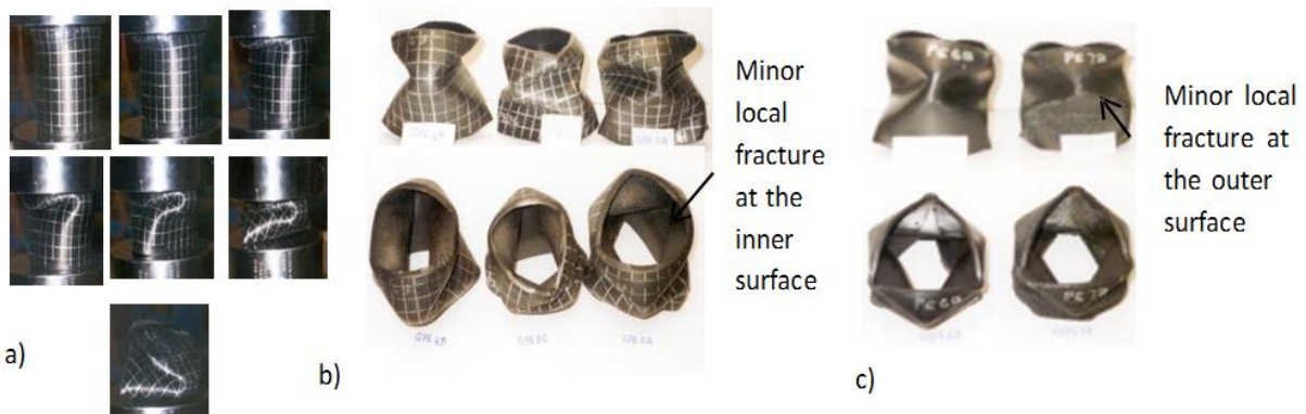
Figure 8 a) Collapse progress, b) Collapse mode of the GPE 4 and GPE 5 ( V_f 5%) and c) Collapse mode of the HDPE 6 and MDPE 7 (non fibre)
