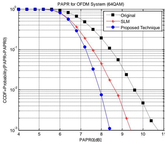
**Figure 4** Comparison of the PAPR reduction in 64 QAM
