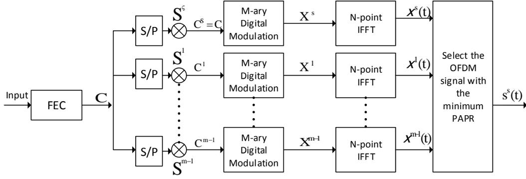
Figure 2 Block Diagram of the proposed technique in OFDM System
