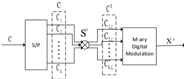
Figure 1 Circulant shift of codeword sub-blocks
