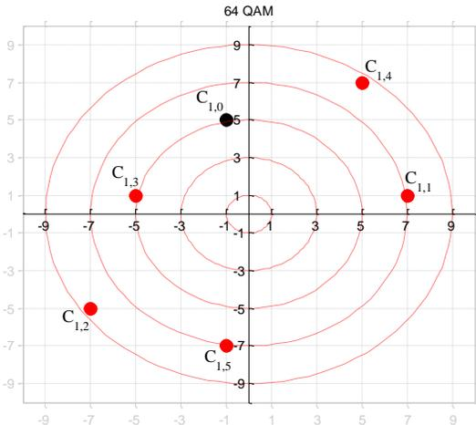
Figure 3 Example 1 of codeword shift for 64 QAM Constellation
